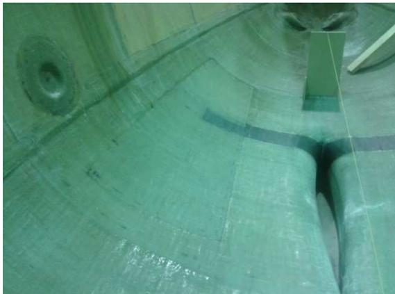
An encapsulated keel, again, has its proponents, but as an engineered solution it only really skirts the issue. An encapsulated keel adds buoyancy volume of GRP reducing the effect of the ballast, in a kind of self-defeating way. However, the fact that an encapsulated keel has continuous structure from fin to hull does appeal. In order to adopt this aspect of good design, the G35 has been
