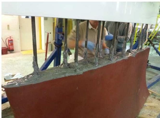
the lead fin, through bonded compression tubes all the way to the top of the stub, and secured above the inner structural laminate. Structurally, the result is effectively a dual fixing. The stub is an exact match of the lead fin section, and is faired to a seamless finish. Why go to all this trouble? After all, it's a man-hour intensive solution. Well, this solution is the best of many worlds:
